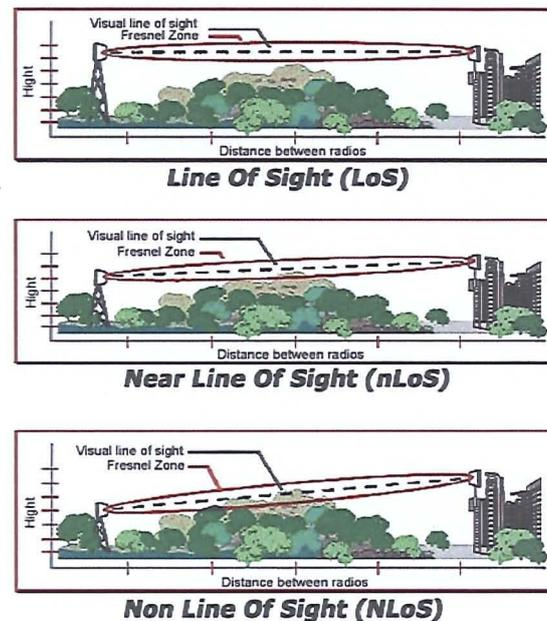
Fig. 22. Diagram of how line of sight (LOS) connection operates in a WiFi network (Accessed 10.10.06. Available at: <http://www.air-stream.org.au/los>).
