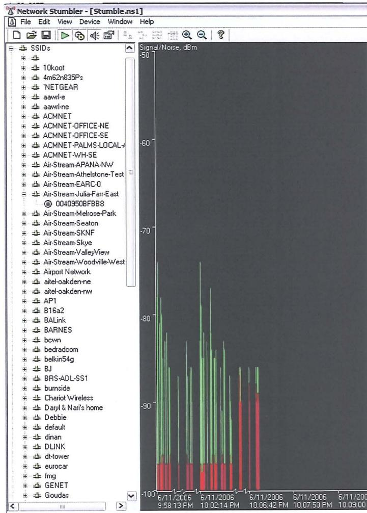
Fig. 39. Screenshots from NetStumbler on the Air-Stream website illustrating a textual and graphic display of wireless 'noise' (Accessed 15.06.08, Available at: [http://www.air-stream.org.au/stumbling\\_software](http://www.air-stream.org.au/stumbling_software)).
