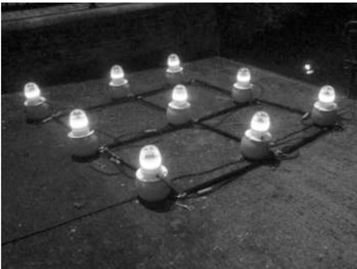
Figure 2: the 3 x 3 buoy Net Work prototype
