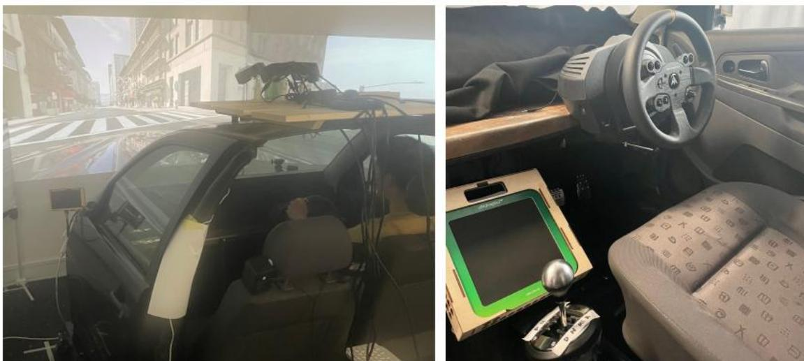
*Figure 3.9. Driving simulator setup, internal and external.*
